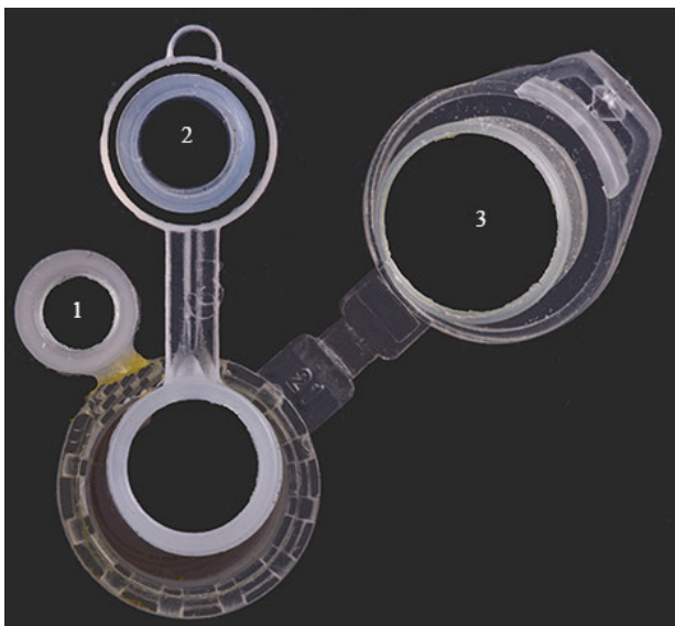
Figure 1. Inner diameters (ID) of caps of a: 1, genitalia vial (4 mm ID); 2, 1 mL storage tube (4.8 mm ID); 3, 1.5 mL microcentrifuge tube (8 mm ID).
