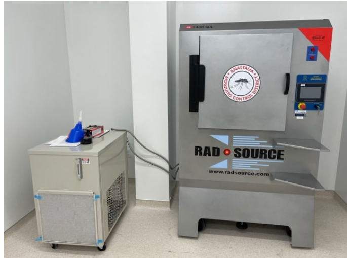
Fig. 2. Radiation machine for irradiating mosquitoes at AMCD's mass rearing facility, St. Augustine, Florida.
